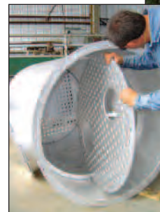
Installing the top splash plate. Large holes accept the chimneys
