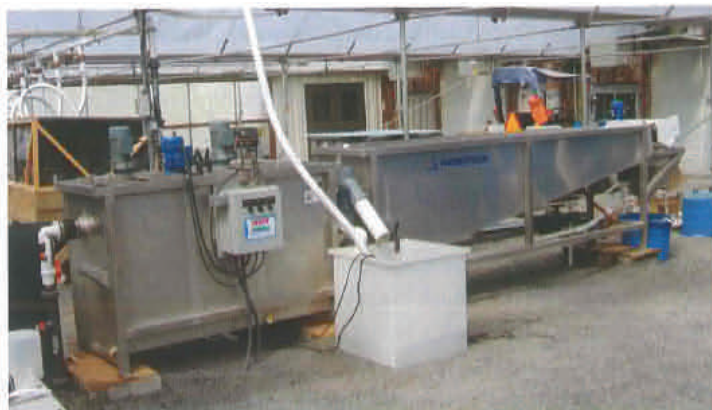
(above) Hydretech Belt Filter System – coagulation/flocculation tank and belt filter. Photos courtesy James Ebeling, The Conservation Fund Freshwater Institute
