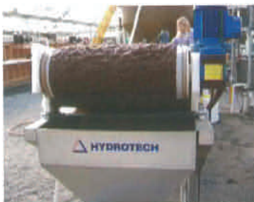
Thickened waste from a conventional microscreen drum filter with coagulation and flocculation aid, alum and polymer.
