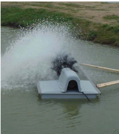
2 hp WaterTek paddlewheel aerator in action
