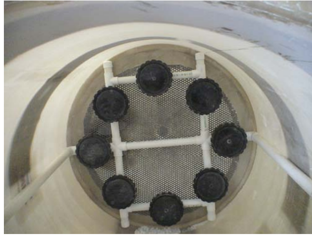
Go Fish GA – Vertical IMF Biofilter with Air Grid and Media Screen – 6 systems (60-180 gpm), 15-75 ft 3 media (0.42-2.1m 3 )
