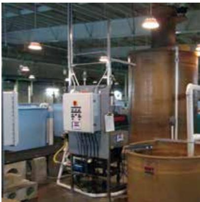
The **Vertical IMF** was developed to deliver compact modular filtration when clients require a smaller footprint which can accommodate taller systems.
